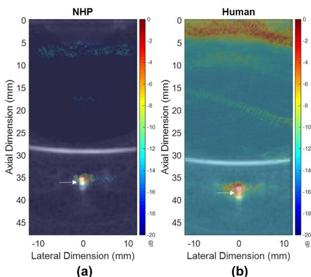
**Fig. 4.** Transcranially-acquired PCI with overlaid B-mode images acquired of the channel phantom without skull interference for the (a) NHP skull, and (b) human skull, utilized to determine RFS. White arrows denote the center of the channel phantom on B-mode acquisitions.
