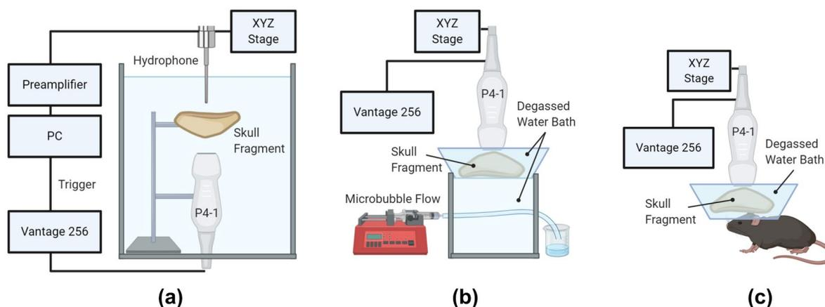
**Fig. 1.** Experimental setup for (a) transcranial pressure attenuation measurements, (b) *in vitro* PCI RFS calculations and (c) *in vivo* synchronous TUS-mediated BBB opening and PCI. Figure created using Biorender.
